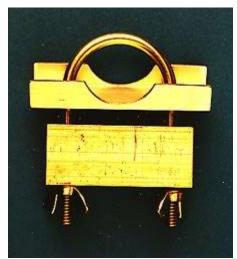
Photo 2--Machined clamp to match 1¼ inch mast.
